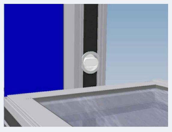
• Close the louvre blade by hand, align it and push the clamp upwards (on the driven side) with slight pressure. Keeping the clamp in position, tighten both stud bolts firmly.
